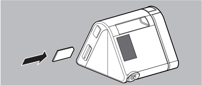
1. Push the SD card into the SD card slot until you hear it engage. The SD card symbol
