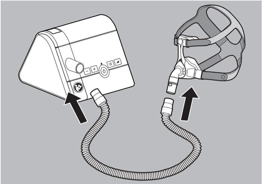
3. Push breathing tube onto the device outlet port.
