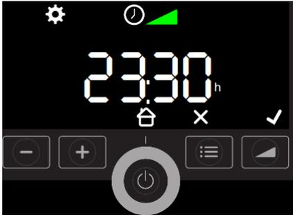
The keys of the device may have different functions. If there is a symbol above the key in the display (e.g. ✓ above the softSTART key), the key adopts the function of the symbol in question. If there is no symbol above the key (e.g. in the case of the + key), the key retains its original function.
