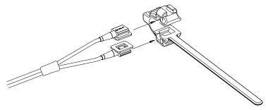
Figure 12-2 Neonate SpO<sub>2</sub> Sensor (1)
