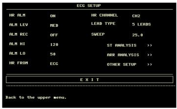
Figure 11-6 ECG Setup Menu
