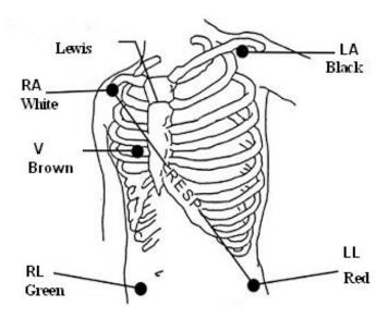
Figure 11-1 Electrode Placement for 5-lead Set
